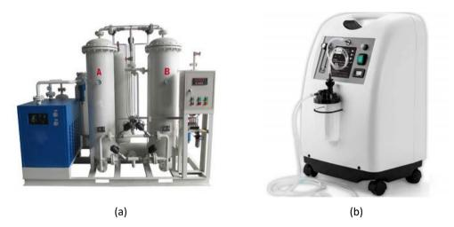
Figure 4. Example of (a) oxygen generators and (b) oxygen concentrators
